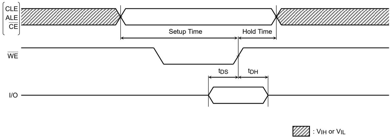
Command Input Cycle Timing Diagram
