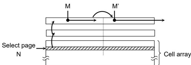
During the serial data output from the Data Cache, the column address can be changed by inputting a new column address using the 05h and E0h commands. The data is read out in serially starting at the new column address. Random Column Address Change operation can be done multiple times within the same page.
