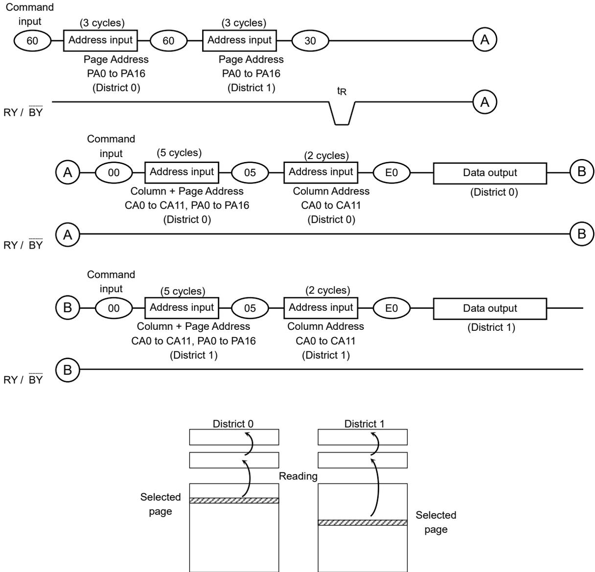
The data transfer operation from the cell array to the Data Cache via Page Buffer starts on the rising edge of  $\overline{\text{WE}}$  in the 30h command input cycle (after the 2 Districts' address information has been latched). The device will be in the Busy state during this transfer period. After the transfer period, the device returns to Ready state. Serial data can be output synchronously with the  $\overline{\text{RE}}$  clock from the start address designated in the address input cycle.
