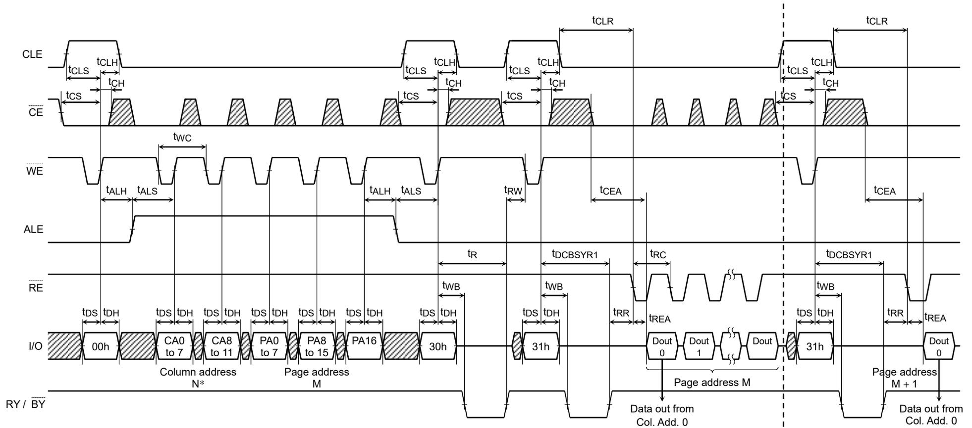
\* The column address will be reset to 0 by the 31h command input.
