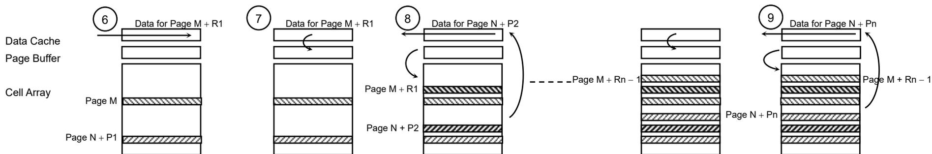
6. Address for Page (M + R1) is input. If the data needs to be changed, changed data is input.
