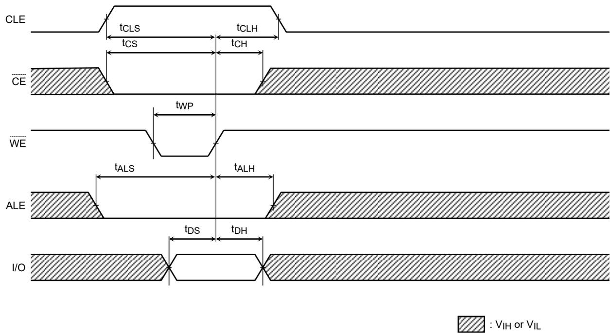
Address Input Cycle Timing Diagram
