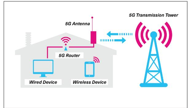
Figure 3: A 5G fixed wireless access configuration
